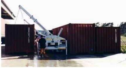
⇒ Much increased efficiency with the ability to move two containers without relocating the Swing Thru
