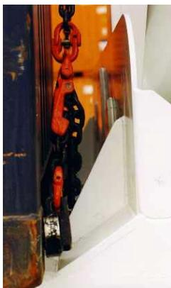
⇒ Speeds the loading of the container by automatically sliding the container into its correct position on the twist locks.
