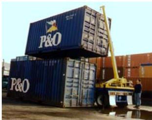
Has the ability to do multiple shifts of containers without having to move the Swing Thru unit
