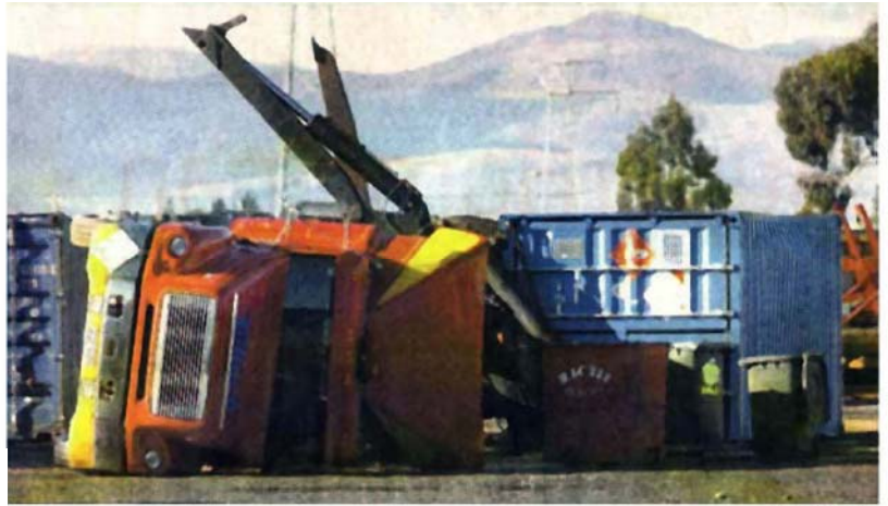
This single-sided side loader overturned while lifting a container, spilling toxic chemicals.
