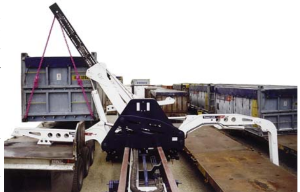
Swing Thru can be positioned between a truck and rail wagon and used as a mobile crane
