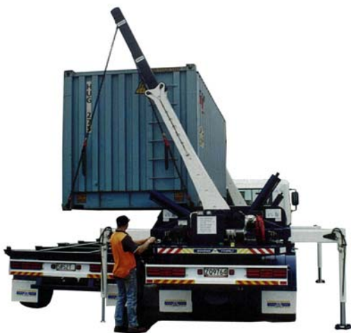
All Swing Thru Double-Sided Container Handling Systems incorporate four-corner stabilisation
