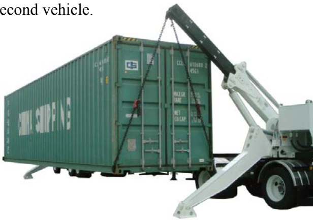
Rapid deploying Swing Thru slam-down legs for fast execution of pick-up-and-carry operations
